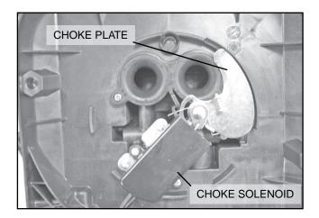
Figure 23. Solenoid Energized, Choke Open 12-20 kW Units
